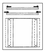
Figure 3-3. Turning the Steel Rails Increases Spacing Between Them
