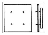
Figure 3-1. Screws Attach Mounting Plates to Filter Holder
